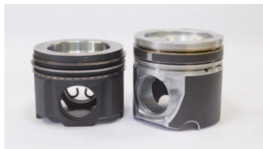
Steel piston (left) compared with a conventional aluminum piston.
